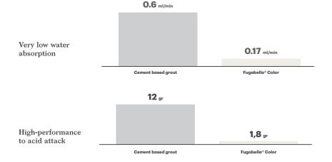
The purity of the materials employed, the use of specific natural additives, result in superior protection from water.
