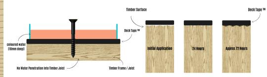
Completely **Self Sealed** When Fastener Is Driven Through The Deck Tape ™
