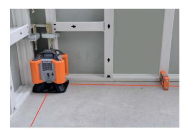
**Well-designed.** Numerous innovative ideas went into the development of the LINUS<sup>1</sup> HV. The housing dimensions of the laser and ACCEPTOR<sup>Line</sup> laser receiver are perfectly matched. The distance between the vertical laser plane and the edge of the LINUS<sup>1</sup> HV is identical to that between the edge and zero line of the laser receiver.
