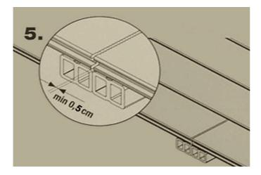
Note: When calculating the end-to-end gap, add 2mm for every 10°C difference between the highest temperature the decking will be exposed to, and the temperature at installation.
