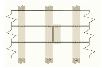
For the first board, install to the baton as detailed above. For the second board, attach a second board on a second baton/joist – as above diagram.
