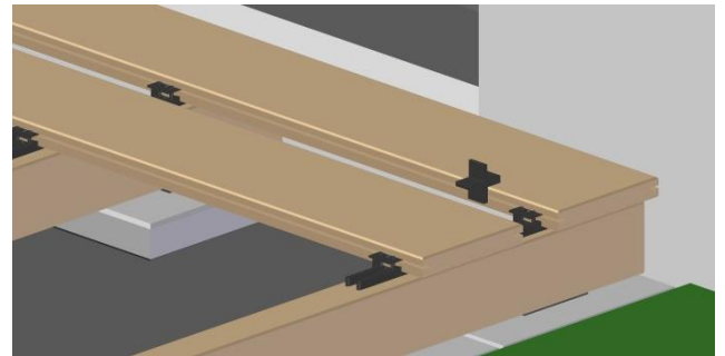
Figure 4 Use the spacer to ensure correct gap
