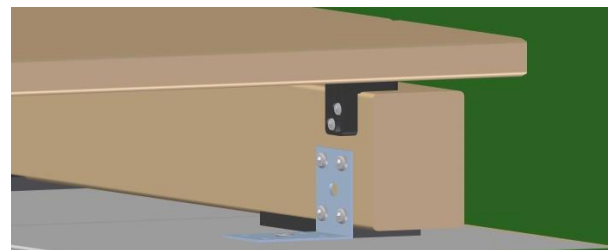
Figure 8 Screw the clip to the base construction
