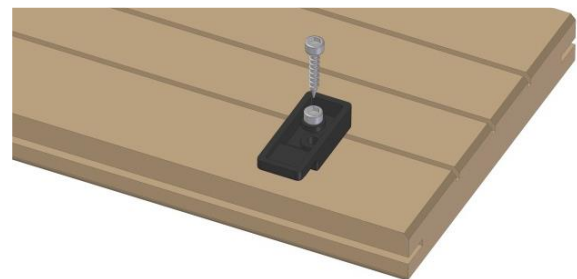
Figure 2 Mount starting clips on the underside of the first board
