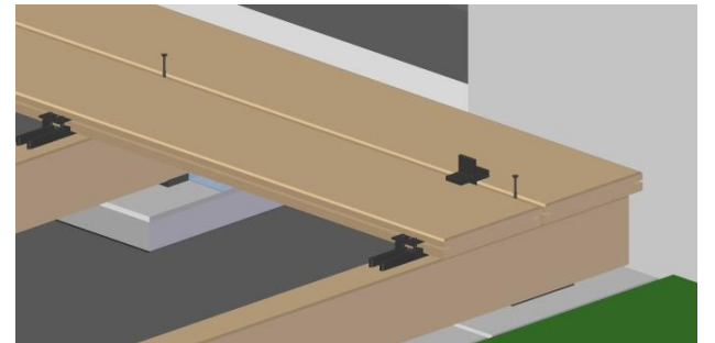
Figure 5 Do not screw the terrace clips in place until the subsequent board is properly in place
