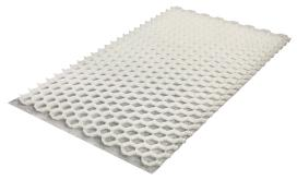
Both the large sheet (2400x1150mm) and the small sheet (1150x800mm) come with a 50gsm non-woven weed membrane heat welded to the underside of the grid. This not only prevents weed growth from beneath the surface, but also prevents the gravel from migrating under the cell wall and into the sub base over time.
