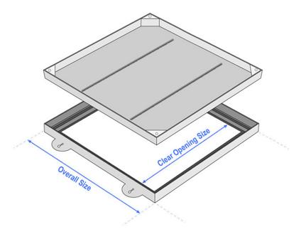
Whether your manhole is square or round, the same principal applies. You should measure the distance between the inside walls of the manhole.
