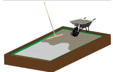
Fill the grid with your chosen aggregate either using a wheelbarrow or direct from a truck. Ensure the truck does not drive on unfilled cells. CORE Drive is designed to be covered by a 10-15mm dressing layer of aggregate making the grid virtually invisible.
