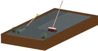
To install CORE Drive over an existing old gravel driveway, tarmac or concrete surface you first need to clear the area of weeds and any loose material.
