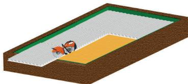
Install the grid starting from one corner and working your way out with the membrane facing down. Ensure to connect all available clips on all four sides of the sheet and to underlap the membrane where possible. Cut to shape using a petrol disc cutter or grinder. Please ensure to wear necessary PPE for the equipment being used.
