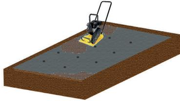
Repair the surface if there are any large dips or pot holes with a suitable subbase material and recompact the entire area with a roller or vibrating road plate. If installing over tarmac or concrete you may want to drill drainage holes in the surface to allow water infiltration.
