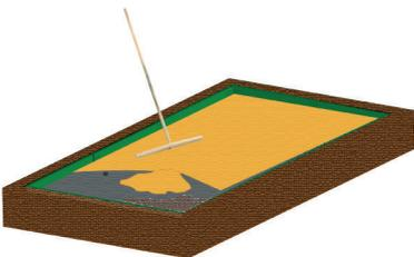
Cover the entire area with a 5-10mm bedding layer of sharp sand and compact. This layer will help to eliminate any minor undulations you may have in your subbase, it also helps to protect the membrane attached to the underside of the grid from the subbase material.
