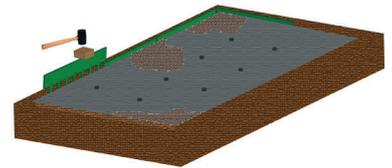
Install a suitable edging around all open sides. This can be a tanalised wooden edging; block paviours; granite setts; concrete path edgings or our very own flexible metal edging (CORE Edge).
